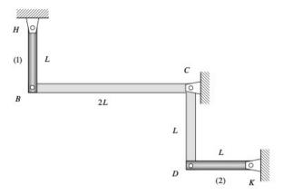
Identical elements (1) and (2) (each having a Young's modulus E, coefficient of thermal expansion  $\alpha$  and cross-sectional area A) are connected between ends B and D, respectively, of a rigid, L-shaped bar. The temperature of (1) is *increased* by an amount of  $\Delta T > 0$ , with the temperature of element (2) being held constant.
