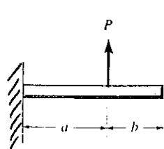
$$v = \frac{Px^2}{6EI}(3a - x) \quad v' = \frac{Px}{2EI}(2a - x) \quad 0 \leq x \leq a$$
