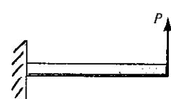
$$v = \frac{Px^2}{6EI}(3L - x) \quad v' = \frac{Px}{2EI}(2L - x)$$
