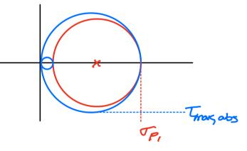
3. If the yield stress of this material is 20 MPa, does the maximum absolute shear stress criterion predict failure?
