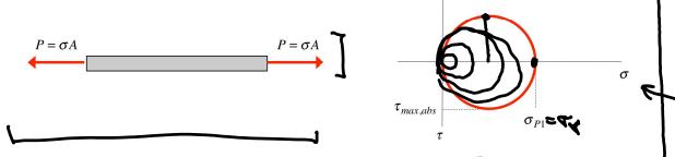
Therefore, from the Mohr's circle for this test, we see that  $\tau_{max} = \frac{\sigma_Y}{2}$  at failure.
