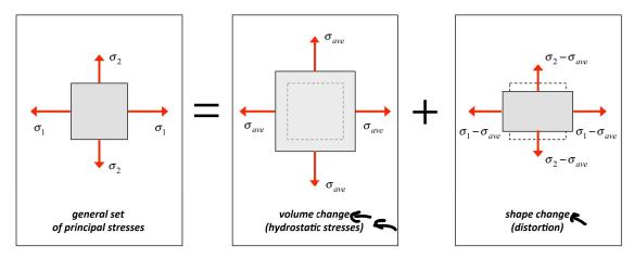
A portion of this energy goes into changing the volume of a stress element, with the remainder going into the change in shape (or "distortion"). The contributions to changes in volume and to distortion are demonstrated in the following figures.
