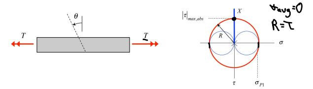
• What is the maximum normal stress in the shaft? On which plane does this stress exist?
