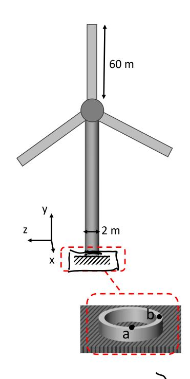
The wind applies a distributed load of 300 N/m on each of three blades that are 60 m long. The rotor assembly and nacelle together weigh ~74 000 kg. The shaft of the windmill is 2 m in diameter at the base and is made of steel that has a thickness of 0.1 m. The weight of the shaft can be neglected compared to the weight of the rotor assembly and nacelle.
