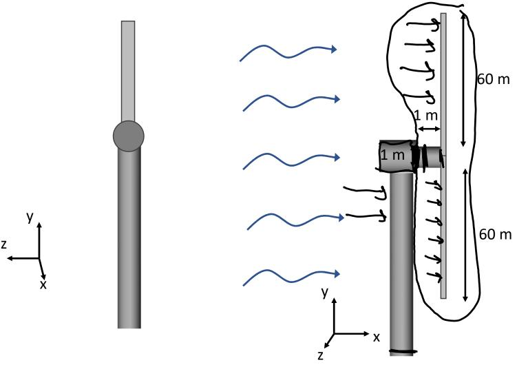
The rotor assembly weighs ~8 000 kg. A distributed force of 300 N/m acts over the blades, which are each 60 m long. Find the stresses at the interface between the hub and the nacelle.
