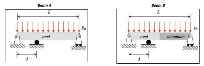
This beam is INDETERMINATE. External reactions and internal resultants are found from both equilibrium considerations and integration of the beam deflection equations, where the latter requires information on the material properties. Therefore, material properties are needed to solve for stresses.
