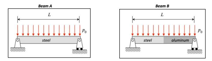
This simply-supported beam is DETERMINATE. External reactions and internal resultants are found directly from equilibrium considerations. Therefore, material properties are not needed to solve for stresses.
