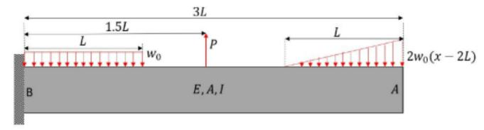
Select the general form that the equation for flexural energy due to bending will take (note that  $f_i(x)$  represents some *continuous* function  $M^2(x)/(2EI)$  for the length of integration):
