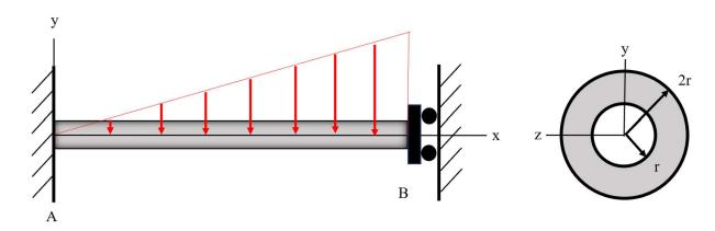
A circular beam of length L, Young's modulus E, outer radius 2r, and inner radius r is supported by a fixed end at A and a roller at B. A linearly varying line load  $p(x) = -p_o \frac{x}{L}$  acts on the entire length of the beam  $\left(p(L) = -p_o \left[\frac{N}{m}\right]\right)$ . Solve the following using the  $2^{nd}$  order integration method.
