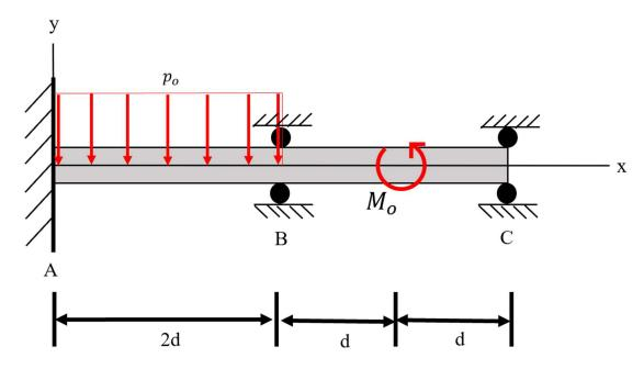
A beam of length L=4d, Young's modulus E, and  $2^{nd}$  area moment I is supported by a fixed end at A and rollers at B and C. A line load  $p_o\left[\frac{N}{m}\right]$  acts on the beam from A to B, and a moment  $M_o$  acts at location 3d. The value  $M_o = p_o d^2[Nm]$ . Complete the following questions using superposition. Note: you can use the tables in the Appendix of your book as a reference.
