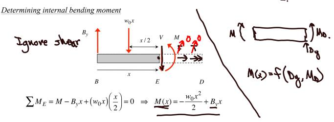
Strain energy in beam (ignoring contributions from shear stress/strain)
