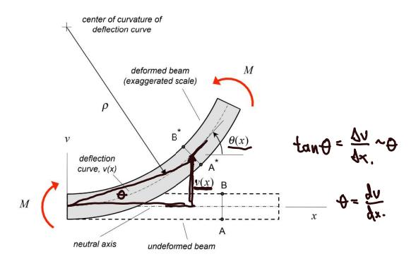
In this figure,  $\theta(x)$  is the angle of rotation of the cross section of the beam and  $\rho(x)$  is the radius of curvature of the deflection curve v(x). From basic calculus,  $\theta(x)$  and  $\rho(x)$  can be expressed in terms of the deflection curve v(x) as:
