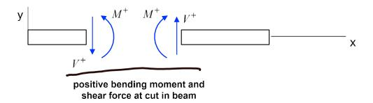
Sign conventions for *external* loadings on beams:
