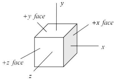
The three components of normal stress and the six components of shear stress shown on the body on the previous pages all correspond to positive quantities. These components on the positive faces, along with those on the negative faces, are shown on the stress cube below, where a “primed” quantities (e.g.,  $\sigma'_x$  and  $\tau'_{xy}$ ) are those components on the negative faces.
