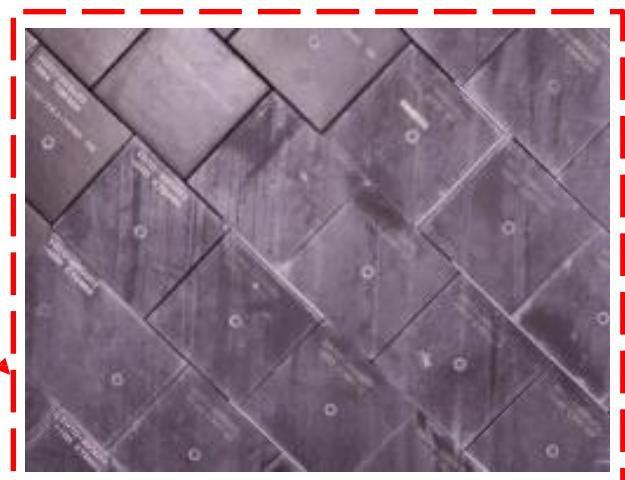
During re-entry, the space shuttle locally experiences temperatures up to 1500 °C. The heat-protection tiles on the surface of the shuttle are designed to have a small thermal expansion coefficient, but gaps are still left between tiles to allow thermal expansion.
