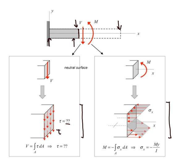
We have seen that the normal stresses due to the bending moment M are linearly distributed over the cross section, with maximum magnitudes of normal stress occurring on the outer fibers of the beam and with zero normal stress at the neutral axis (the neutral axis passing through the centroid of the cross section).
