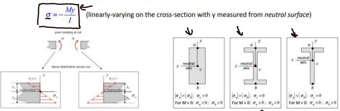
ullet Where on the cross-section is the flexural stress the greatest? $\Upsilon$
