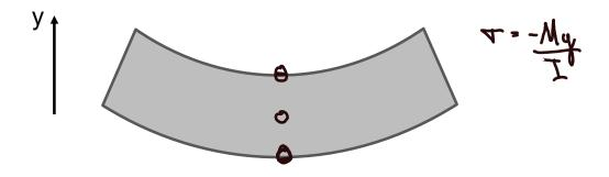
Beams: Flexural and shear stresses
