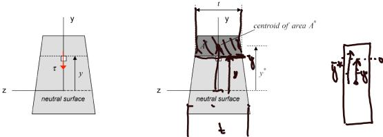
Consider the cross section shown above. We desire to know the shear stress  $\tau$  acting on a stress element at a distance of y from the neutral surface. This shear stress along the axis of symmetry (the y-axis) can be expressed as:
