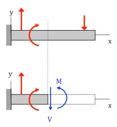
• Shear force/bending moment equation:
