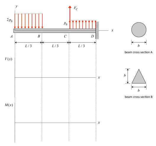
Determine the deflection of the beam loaded as below using superposition.
