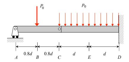
Draw the shear force and bending moment diagrams in the plot axes below for the loaded beam shown.
