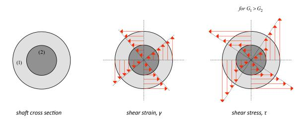
Stress elements on a cut made perpendicular to the member axis are as shown.
