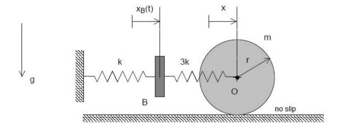
Use the following parameters in your analysis: m = 80 kg, k = 640 N/m, r = 0.25 m, b = 0.16 m, and  $\Omega = 10$  rad/s.
