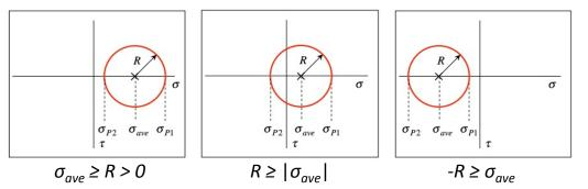
Subsequent rotation about the *n*-axis produces a Mohr's circle between 0 and  $\sigma_{P2}$  on the  $\sigma$ -axis. Similarly, an alternate rotation about the *t*-axis produces a Mohr's circle between 0 and  $\sigma_{P1}$  on the  $\sigma$ -axis.
