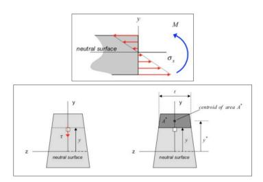
The process for determining these components of stress in *determinate* beams is the following:
