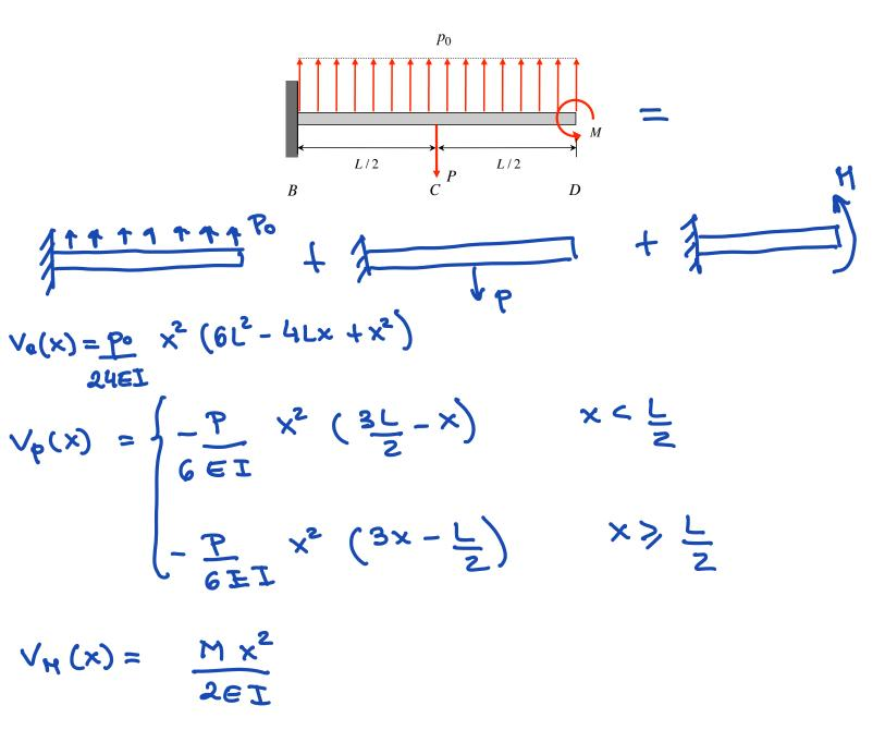
Determine the load carried by rod BD using superposition. The beam has a flexural rigidity of EI. Rod DB is made of a material with a Young's modulus of E, cross-sectional area of A and length L.
