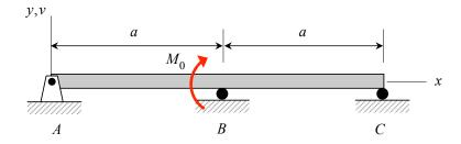
Consider the beam below with propped cantilevered supports and a couple applied at point B. The beam has a square cross-section with dimensions of  $h \times h$ .
