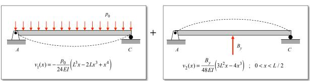
The internal bending moment in the beam is found from, for 0 < x < L/2:
