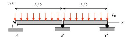
Consider the beam below with a pin support at A and roller supports at B and C. The beam has a circular cross-section with a diameter of d. The material making up the beam has a Young's modulus of E.
