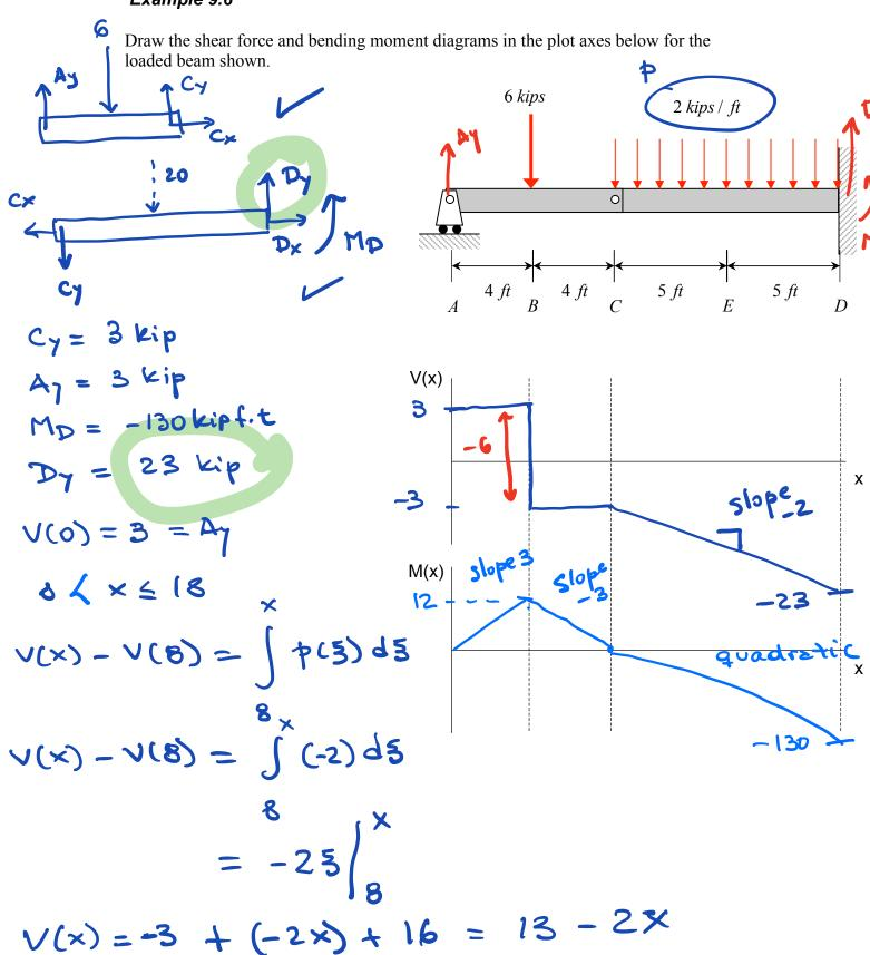
Beams: Bending moments and shear forces
