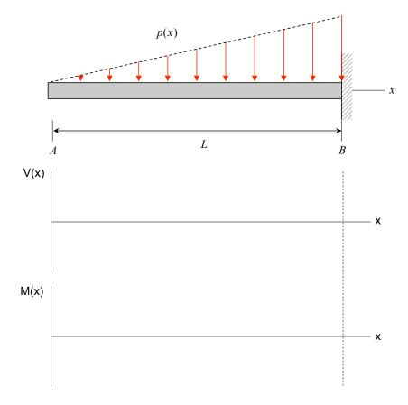
Use the following three methods to draw the shear force and bending moment diagrams in the plot axes below for the loaded beam shown: i) direct use of FBDs and equilibrium, ii) formal integration, and iii) integration by inspection. Clearly indicate the values of V and M at the labeled points as well as any maximum/minimum values. Please provide details on your work. Use  $p_0 = 2kN/m$ , L = 3m,  $P_0 = 2kN$  and  $M_0 = 5kN \cdot m$ .
