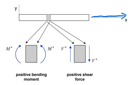
When making a cut through a cross section of the beam, the positive sign conventions for the bending moment and shear force are as shown below:
