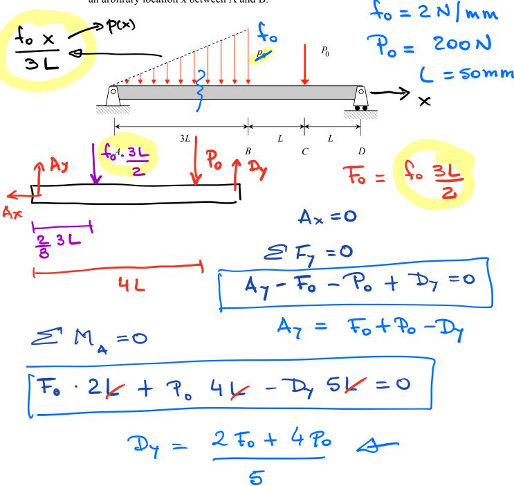
$$F_0 = f_0 \cdot \underbrace{3L}_{2} = \underbrace{2N}_{mm} \underbrace{3.50mm}_{2}$$
