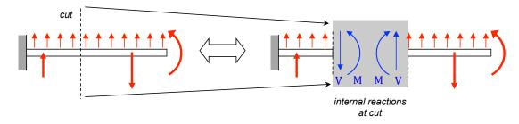
• V and M are force/couple resultants of the normal and shear stresses acting on the face of a cross section.
