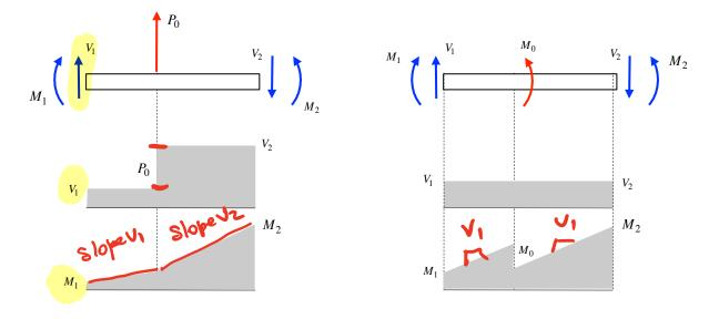
Beams: Bending moments and shear forces
