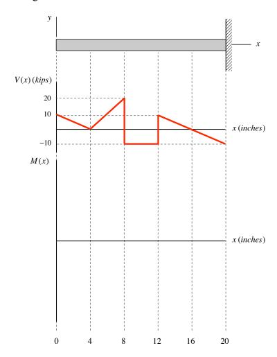
Draw the shear force and bending moment diagrams in the plot axes below for the loaded beam shown.
