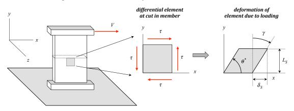
Shear strain deformations produce skewing in a rectangular-shaped element: the angle between adjacent sides changes from  $\pi/2$  to  $\theta^*$ . Here, we will define the shear strain as  $\gamma$  representing this change in angle:
