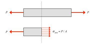
Since the axial load throughout the rod is *P*, we can write down that the average axial stress is the axial force divided by the cross-sectional area:
