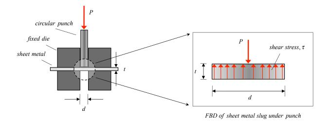
With a small clearance between the punch and the inner diameter, the sheet metal experiences a state of direct shear. Here, we can calculate the shear stress acting on the circumference of the punch slug as:
