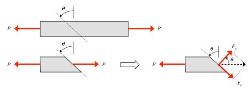
As a result of this cut, we see two changes. First, the axial load now has both normal and tangential components on the cut face of:
