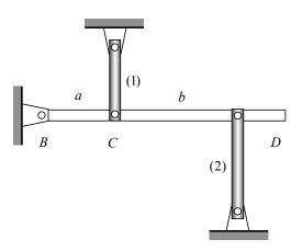
$$\theta = angle \ of \ rigid \ bar \ rotation = \frac{e_1}{a} = -\frac{e_2}{b} \implies e_1 = -\left(\frac{a}{b}\right)e_2$$
