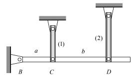
$$\theta = angle \ of \ rigid \ bar \ rotation = \frac{e_1}{a} = -\frac{e_2}{a+b} \implies e_1 = -\left(\frac{a}{a+b}\right)e_2$$
