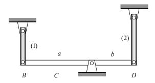
$$\theta = angle \ of \ rigid \ bar \ rotation = \frac{e_1}{a} = \frac{e_2}{b} \ \Rightarrow \ e_1 = \left(\frac{a}{b}\right)e_2$$
