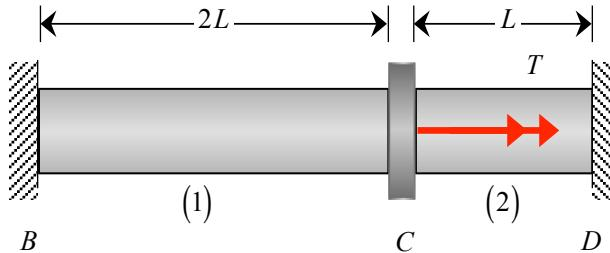
Consider an axial torque  $T$  acting on a shaft with a circular cross section. To solve for torque in each element, use the four-step plan:
