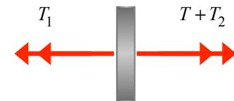
2. *TORQUE/ROTATION*:  $(2) \Delta\phi_1 = \frac{T_1(2L)}{GI_P}$
