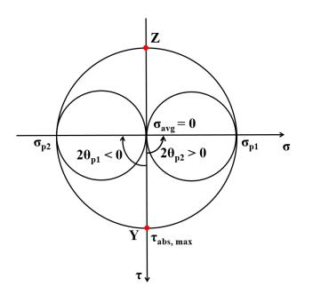
Principal stress:  $\sigma_{p_1} = 32.59 \text{ kPa}$ ,  $\sigma_{p_2} = -32.59 \text{ kPa}$ Principal angle:  $= \theta_{p_1} = +45^\circ, \theta_{p_2} = -45^\circ$ Maximum in plane shear stresses:  $\tau_{inplane,max} = 32.59 \text{ kPa}$ Absolute shear stress:  $\tau_{max,abs} = 32.59 \text{ kPa}$ <u>Case (b):</u>
