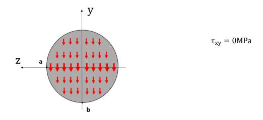
Normal Stress Distribution due to bending moment 1  $(M_y)$  at point 'a':
