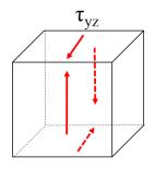
Since,  $\sigma_z = 0$ ,  $\tau_{yx} = \tau_{xz} = 0$ , the yz plane is the plane corresponding to the state of plane stress.
