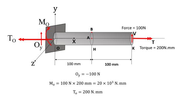
Making a cut at H and finding the internal resultant force, moment and torque we have:
