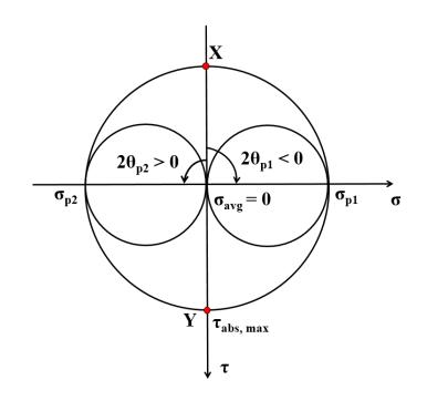
Principal stress:  $\sigma_{p_1} = 32.59 \text{ kPa}$ ,  $\sigma_{p_2} = -32.59 \text{ kPa}$ Principal angle:  $= \theta_{p_1} = -45^\circ, \theta_{p_2} = 45^\circ$ Maximum in plane shear stresses:  $\tau_{inplane,max} = 32.59 \text{ kPa}$ Absolute shear stress:  $\tau_{max,abs} = 32.59 \text{ kPa}$
