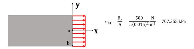
Stress distribution due to Shear force 1 (B<sub>y</sub>) loading at point 'b':
