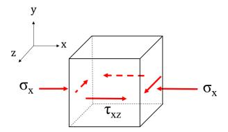
$\sigma_x = 3.77 \text{ MPa}$   $\tau_{xz} = \ 0.0377 \text{ MPa} = 37.7 \text{ kPa}$
