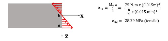
Normal Stress Distribution due to bending moment 2 (Mz) at point 'b':
