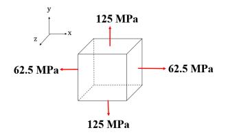
Since,  $\sigma_z = 0$ ,  $\tau_{yz} = \tau_{xz} = 0$ , the xy plane is the plane corresponding to the state of plane stress.
