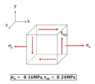
Since,  $\sigma_z=0, \ \tau_{yz}=\ \tau_{xz}=0$  , the  $xy\,$  plane is the plane corresponding to the state of plane stress.
