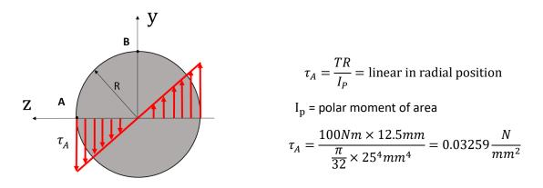
There are no normal stresses acting on the point A,  $\sigma_x = 0$ ,  $\sigma_y = 0$  and the only shear stress acting is in the xy plane,  $\tau_{xy} = 32.59$  kPa
