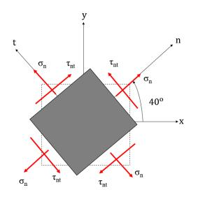
The rotation of the inclined plane is =  $40^{\circ}$  (C. C. W), the point 'N' on the Mohr's circle will be at an angle of  $80^{\circ}$  (C. C. W) from point 'X'.
