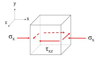
Principal stress:  $\sigma_{p_1} = 10.33 \text{ MPa}$ ,  $\sigma_{p_2} = -43.57 \text{ MPa}$ ,  $\sigma_3 = 0 \text{ MPa}$ Maximum in plane shear stresses:  $\tau_{inplane,max} = 26.95 \text{ MPa}$ Absolute shear stress:  $\tau_{max,abs} = 26.95 \text{ MPa}$
