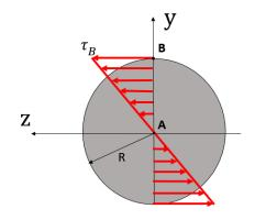
$$\tau_{B} = \frac{T_{H}R}{I_{P}} = \text{linear in radial position}$$
