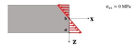
Normal Stress Distribution due to bending moment 2  $(M_z)$  at point 'b':
