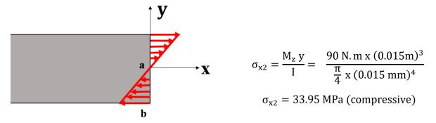
State of stress at point'b':  $\sigma_x = \sigma_{x1} + \sigma_{x2} = 33.24 \text{ MPa} \text{ (compressive)}$   $\sigma_y = 0 \text{ Mpa}$   $\sigma_y = 0 \text{ Mpa}$   $\tau_{xy} = 0 \text{ MPa}$   $\tau_{yz} = 0 \text{ Mpa}$  $\tau_{zx} = 21.22 \text{ Mpa}$
