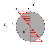
$$\begin{split} \tau_B &= \frac{TR}{I_P} = \text{linear in radial position} \\ I_p &= \text{polar moment of area} \\ \tau_B &= \frac{100\text{Nm} \times 12.5\text{mm}}{\frac{\pi}{32} \times 25^4\text{mm}^4} = 0.03259 \frac{\text{N}}{\text{mm}^2} \end{split}$$
