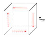
Since,  $\sigma_z = 0$ ,  $\tau_{yz} = \tau_{xz} = 0$ , the xy plane is the plane corresponding to the state of plane stress.
