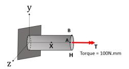
Internal resultant forces include only the torque.
