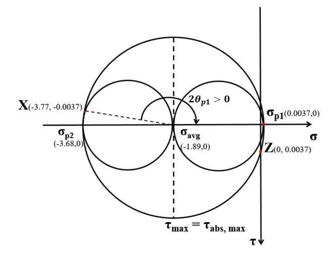
Principal stress:  $\sigma_{p_1} = 0.0037 MPa$ ,  $\sigma_{p_2} = -3.77 \text{ MPa}$ ,  $\sigma_3 = 0 \text{ MPa}$ Principal angle:  $= \theta_{p_1} = 90.57^o$ ,  $\theta_{p_2} = 0.57^o$ Maximum in plane shear stresses:  $\tau_{inplane,max} = 1.8854 \text{ MPa}$ Absolute shear stress:  $\tau_{max,abs} = 1.8854 \text{ MPa}$
