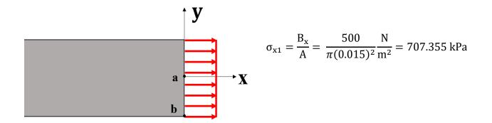
Stress distribution due to Shear force 1  $(B_y)$  loading at point '*a*':
