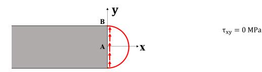
Stress distribution due to torsional loading at point B:
