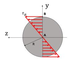
$\tau_{xy} = \frac{T_H R}{I_P} = \text{linear in radial position}$   $I_p = \text{polar moment of area}$   $\tau_{xy} = 0 \text{MPa}$
