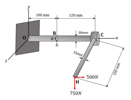
Consider the elastic structure shown in the figure, where a force equal to 500 N i - 750 N j is applied at the end of the segment CH parallel to the z-axis.
