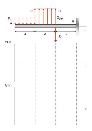
Draw the shear force and bending moment diagrams in the plot axes below for the loaded beam shown.
