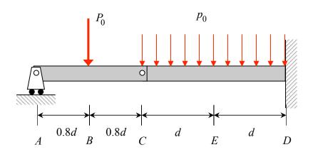
Draw the shear force and bending moment diagrams in the plot axes below for the loaded beam shown.
