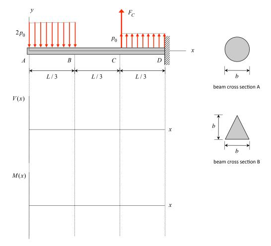
Determine the deflection of the beam loaded as below using superposition.
