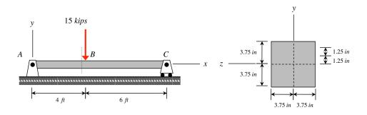
Beam AD is loaded as shown.
