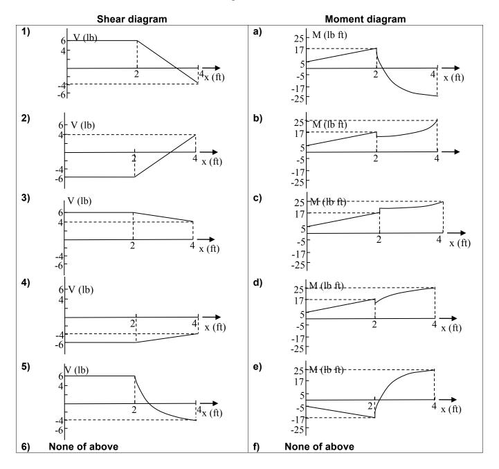
Determine the shear force and bending moment diagrams in the plot axes below for the loaded beam shown. Clearly indicate the values of V and M at the labeled points as well as any maximum/minimum values. Please provide details on your work. Use  $p_0 = 20lb / in$ , a = 2in and  $P_0 = 40lb$ .
