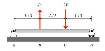
Consider the indeterminate beam shown below, where the beam is made up of a material having a Young's modulus of E and a cross-sectional second area moment of I. For this beam, determine its deflection at the midpoint H. Use the superposition approach with known beam deflection solutions.
