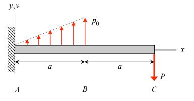
Determine the deflection curve v(x) for the beam shown below.
