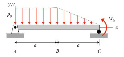
Determine the deflection curve v(x) for the beam shown below.
