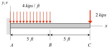
Determine the deflection curve v(x) for the beam shown below.
