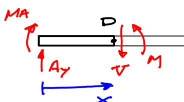
$$\therefore V_B = \frac{1}{EI_1} \int_0^{L_1} (A_y x + M_A) (-x + L_1) dx + \frac{f_s}{G.A_1} \int_0^{L_1} (A_y) dx \quad (3)$$
