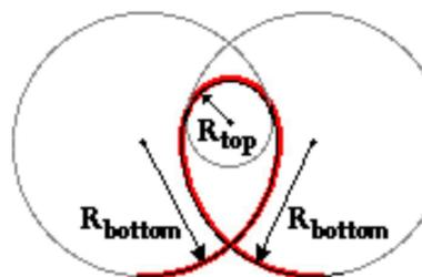
The radius at the bottom of a clothoid loop is significantly larger than the radius at the top of the clothoid loop.
