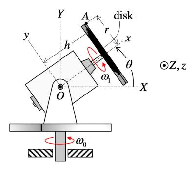
Use the following parameters in your analysis:  $\omega_0=1$  rad/s,  $\theta=30^\circ$ ,  $\dot{\theta}=0.3$  rad/s,  $\omega_1=60$  rad/s, h=0.15 m, and r=0.1 m.
