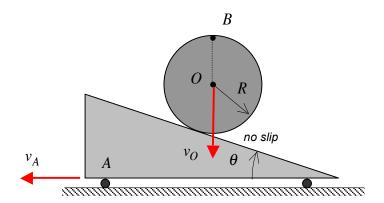
Use the following parameters in your analysis: R=1.5 ft,  $v_A=30$  ft/s and  $\theta=20^\circ$ .
