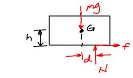
The homogenous bar shown is released from rest while in contact with the smooth horizontal surface. Describe in words and with a sketch the path of the center of mass G after the bar is released.
