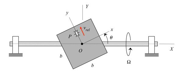
Use the following parameters in your analysis: b=6 in,  $v_{rel}=12$  in/s,  $\Omega=3$  rad/s and  $\dot{\theta}=5$  rad/s.
