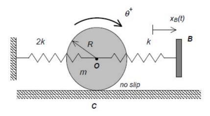
Use the following parameters in your analysis: m = 24 kg, k = 108 N/m, R = 0.2 m, and b = 0.03 m.
