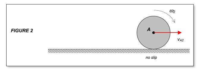
Use the following parameters in your analysis: M = 50 kg, R = 0.5 m,  $\mu_k = 0.3$ ,  $v_{A1} = 5$  m/s and  $\omega_1 = 8$  rad/s.
