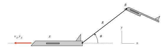
Use the following parameters in your analysis: R = 80 m,  $v_A = 700$  m/s,  $\dot{v}_A = 4$  m/s<sup>2</sup> and  $\theta = 20^{\circ}$  and  $\dot{\theta} = 0.1$  rad/s.
