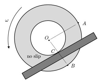
The stepped wheel shown above rolls without slip, in the direction indicated, along an inclined plane. Assuming  $\omega$  is constant, on the drawing above:
