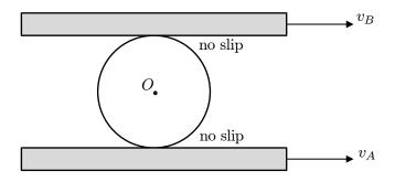
A disk is constrained to roll without slip between two moving surfaces. If each *surface* is moving to the right and  $v_B > v_A$ , determine the following (circle the correct answer):
