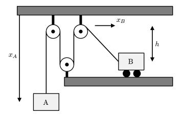
The motion of the two particle system shown above is constrained by an inextensible rope. Circle the correct answer for each of the following questions, assuming  $x_B = 1$  m at the instant shown.
