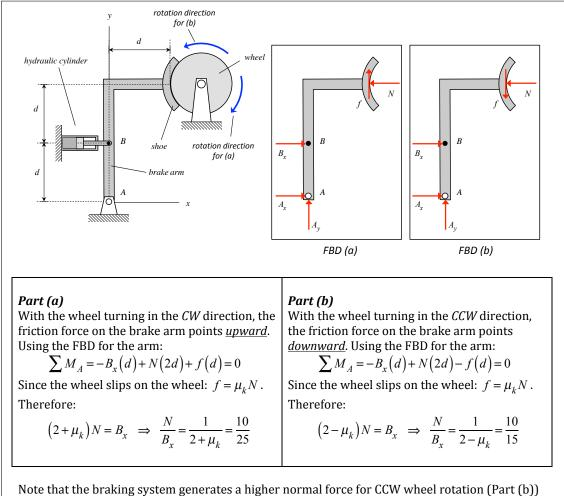
Note that the braking system generates a higher normal force for CCW wheel rotation (Part (b)) than for CW wheel rotation (Part (a)). Therefore, the braking is more efficient for CCW (more friction force for the same piston force  $B_r$ ).
