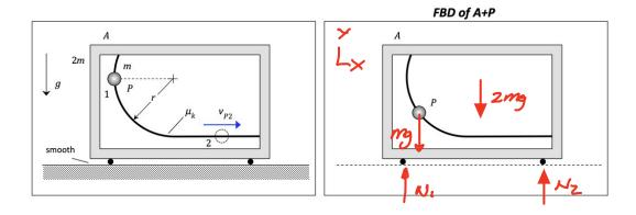
**PART 3A.1:** Using the figure above, draw the free body diagram (FBD) of the combined system of A+P.
