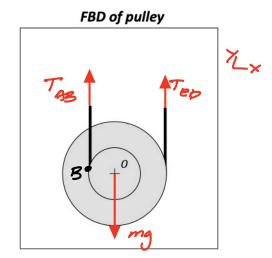
**PART 3B.1:** Using the figure above, draw the free body diagram (FBD) of the stepped pulley.
