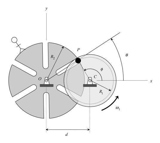
Use the following parameters in your analysis:  $R_1 = 2$  in, d = 4 in and  $\omega_1 = 6$  rad/s.
