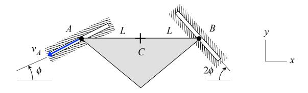
Use the following parameters in your analysis: L=2 ft,  $v_A=15$  ft/s and  $\phi=30^\circ$ .
