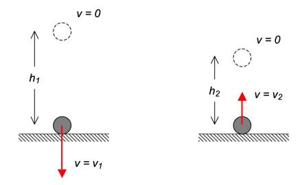
Use the following parameters in your analysis:  $\Delta t = 0.002$  s, m = 15 kg,  $v_1 = 80$  m/s and  $v_2 = 50$  m/s.
