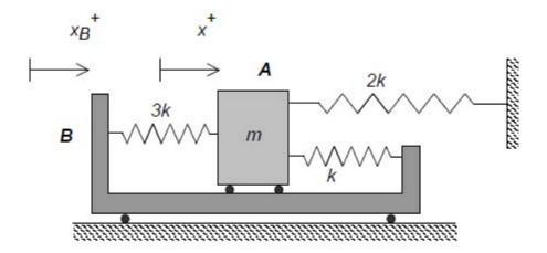
Use the following parameters in your analysis: m=12 kg, k=800 N/m, b=0.1 m, and  $\omega=25$  rad/s.
