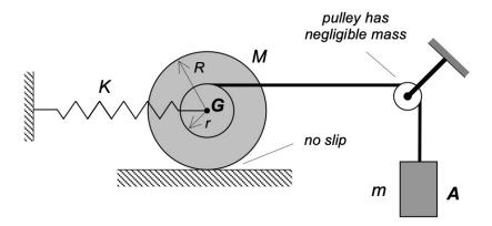
Use the following parameters in your analysis: M=30 kg, m=10 kg, R=0.5 m, r=0.25 m,  $k_G=0.3$  m, K=10 N/m and d=2 m.
