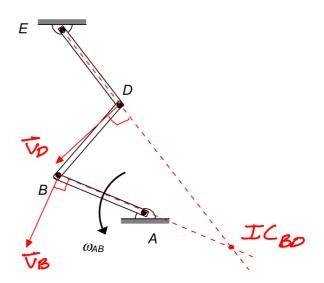
Link AB of the mechanism shown below is rotating counterclockwise when at the configuration shown (when AB and DE are vertical, and BD is horizontal). At this configuration (circle the correct answer):
