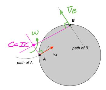
Ends A and B of a thin bar slide on vertical and horizontal surfaces, respectively. At the position shown,  $\theta < 45^{\circ}$ . For this position, circle the answer below that most accurately describes the relative sizes of the speeds  $v_A$  and  $v_B$ :
