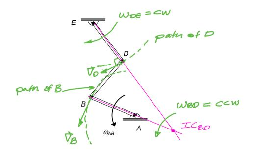
Link AB of the mechanism shown below is rotating counterclockwise when at the configuration shown (when AB and DE are vertical, and BD is horizontal). At this configuration (circle the correct answer):
