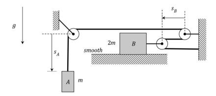
**Given**: Blocks A and B (having masses of *m* and 2*m*, respectively) are connected by an inextensible cable through the cable-pulley system shown above. Consider the pulleys to be ideal (massless and frictionless). Block B is constrained to move along a smooth, horizontal surface, with block A being connected to the free end of the cable.
