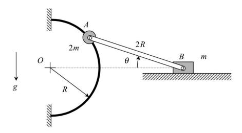
**Given**: Particles A and B (having masses of 2m and m, respectively) are connected by a rod having negligible mass and length of 2R. Particle A is constrained to move on a stationary, vertically-oriented circular guide with a radius of R, whereas particle B moves along a straight, horizontal surface. Consider all surfaces to be smooth. The system is released from rest with rod AB oriented at an angle of  $\theta = \theta_1$  above the horizontal (Position 1).
