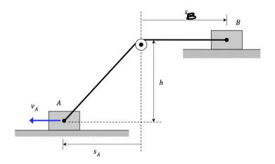
Blocks A and B are connected by an inextensible cable, with the cable wrapped around a small pulley. A moves to the left with a speed of  $v_A$ . Choose the correct response below:
