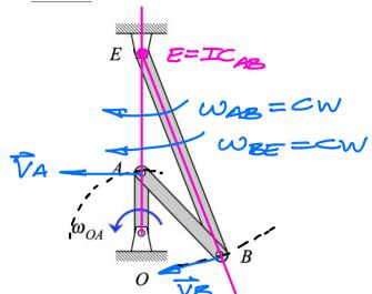
Link OA is rotating in the counterclockwise direction with an angular speed of  $\omega_{OA}$ . At the instant shown, link OA is aligned with line OE, as shown above. Choose the correct responses below (*Hint: Consider the location of the instant center for link AB.*):
