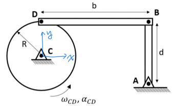
$\overline{W}_{BD} = 0$  (check instant center) Can also be solved as following:  $\overline{BD}: \overline{V}_{B} = \overline{V}_{D} + \overline{W}_{BD} \times \overline{V}_{BD}$  $= -5\hat{\imath} + \overline{W}_{BD}\hat{k} \times \hat{b}\hat{\imath}$
