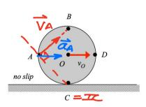
The disk rolls without slipping with its center O having a *constant* speed of  $v_0$ . At the instant shown, A is located directly to the left of O. Circle the correct responses below:
