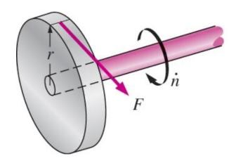
Shaft work for incremental rotation,  $d\theta$
