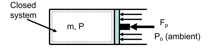
Forces on piston: (for no acceleration of piston)
