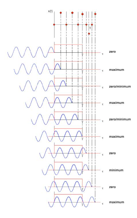
In summary, note that for short pulses, the first maximum in response occurs AFTER the impulse has been turned off, whereas for the long pulses, the first maximum in the response occurs during the action of the impulse. (Here "short" and "long" is relative the natural period of response of the oscillator.)
