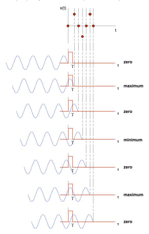
Next consider the <u>long duration pulse</u>. Same process as before. Note that here while the force is "turned on" the minimum value of the response is zero, whereas after the force is turned off the response will be symmetrical about the time axis (the minima being the negative of the maxima).
