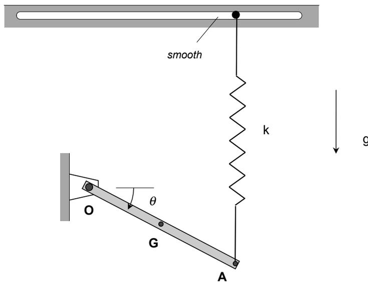
$$T = \frac{1}{2} I_0 \dot{\theta}^2 \quad ; \quad I_0 = I_G + m\left(\frac{L}{2}\right)^2 = \frac{1}{12} mL^2 + \frac{1}{4} mL^2 = \frac{1}{3} mL^2$$
